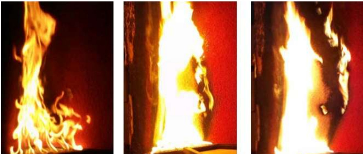
FIG. 6. SAMPLE B2: PICTURES OF FLAME PROPAGATION, DUE TO THE PRESENCE OF DAMAGE, TAKEN AT DIFFERENT TIME STEPS OF THE TEST ( t-t_0 15, 261 and 378 s)
